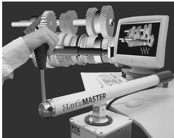
Figure 9: HapticMaster device, from Moog-FCS. Reprint from Thurfjell, McLaughlin, Mattsson, & Lammertse (2002), with permission of Emerald Group Publishing Limited.
