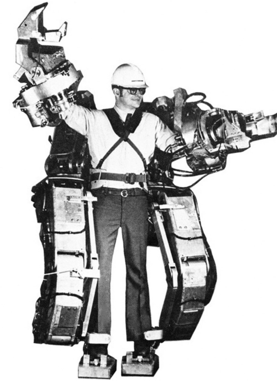
Figure 8: Hardiman from General Electric in 1965 was the first serious attempt to build a powered exoskeleton ("GE Report: The Story Behind the Real 'Iron Man' Suit," n.d.).
