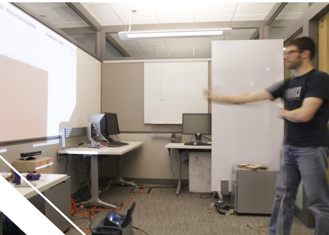
Figure 54: Haptic Kinect setup: the Kinect unit on the left (near the wall), a video projector to display the UI, and me gesturing and testing the haptic box on the right.
