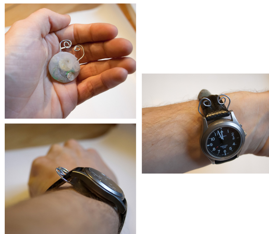
Figure 85: Puce project: a small vibrotactile puck providing haptic notifications in personal communication systems.
